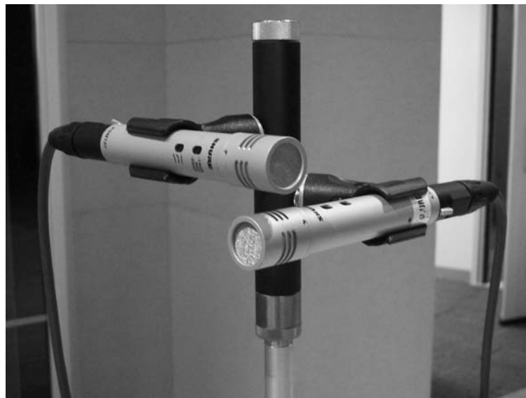
Image 12: Example of “X-Y” stereo miking technique using Shure A27M stereo microphone adapter
