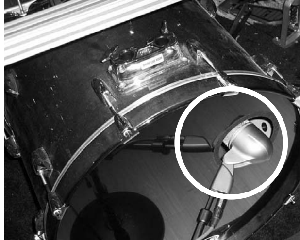
Image 8: Example of bass (kick) drum mic placement
